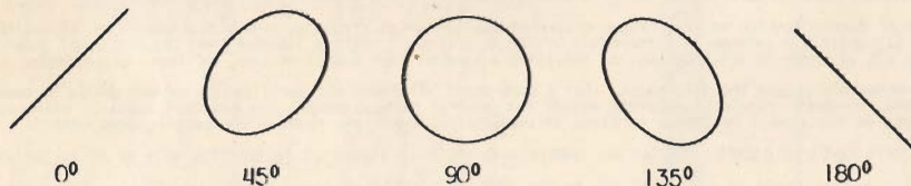
LISSAJOUS FIGURE SHOWING A ONE TO ONE RATIO
